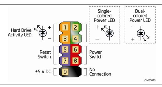
Figure 12. Connection Diagram for Front Panel Header
